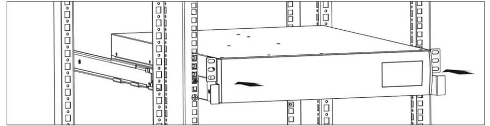
**Step 5:** Fix the UPS in position with 4 screws.
