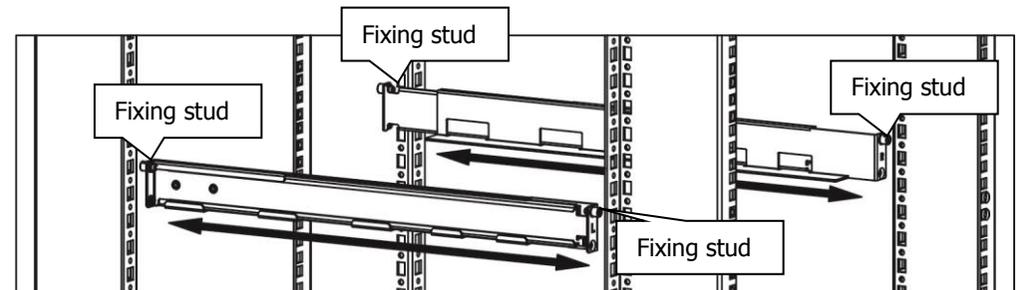
**Step 2:** Use 4 pieces of M6 screws to mount rail sliders into chassis. See chart below:
