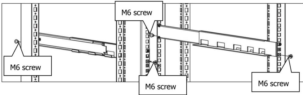
**Step 3:** According to UPS height, put 6 pieces of nuts on proper location.
